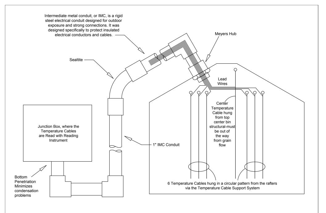
CONDUIT DETAIL FOR HOUSING THE LEADWIRES BETWEEN BIN ROOF & JUNCTION BOX
